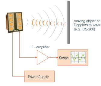
Fig 9: Circuitry for functional test of a IPM 165
