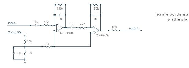
Fig 3: recommended schematic of a LF amplifier with 6...600 Hz bandwidth and 60dB gain
