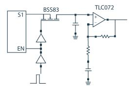
pulsing of a sensor and sample & hold
