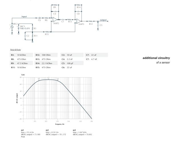
Fig 7: proposal for pre-amplifier circuitry for one channel, 70 dB of gain, 1 kHz bandwidth
