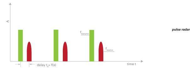
Fig 1: Time-dependent shape of transmit and receive signal of a pulse radar
